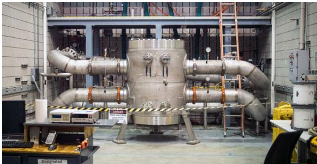
The new world-record magnet connected to cooling water pipes. Some 4,275 gallons of cold water flush through it per minute to keep it cool.
