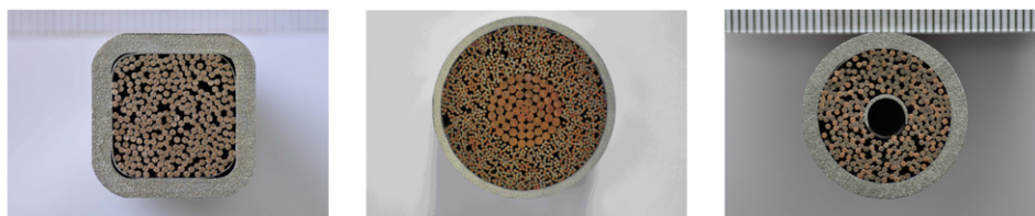
Fig. 1. Cross section of conductor (left: CC, middle: MB, right: CB).
