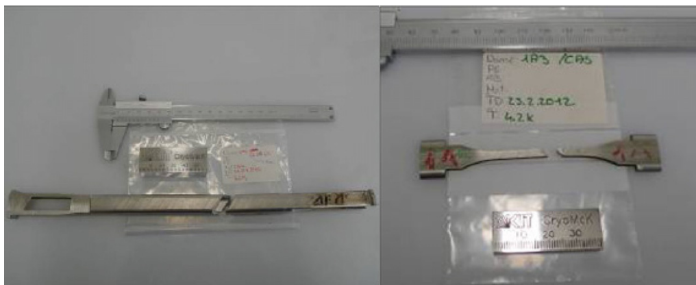
Fig. 8. Fracture surface of CC tensile samples tested at low temperature (<7 K) in KIT.
