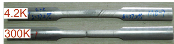
Fig. 7. Fracture surface of MB tensile samples tested in T1CP.
