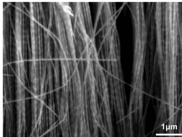
Fig. 1 The FE-SEM images of nanowire released from the AAO template.
