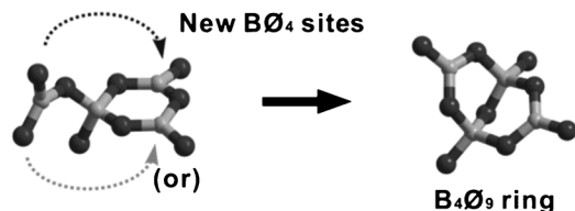
Fig. 10 Schematic of \text{Li}_2\text{B}_4\text{O}_7 crystallization in \text{Li}_2\text{O}\cdot 3\text{B}_2\text{O}_3 melt.
