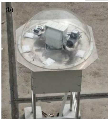
Fig. 7. Schematic drawing (a) and photograph (b) of the GM-DOAS instrument.
