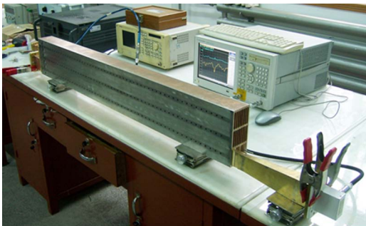
Fig.7 RF test system of the antenna module mock-up (color online)
