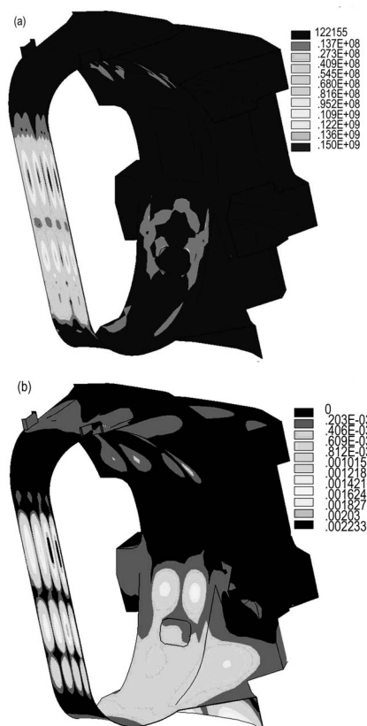
Fig.8 Stress intensity (MPa) and displacements (m) of the ETS under EM load
