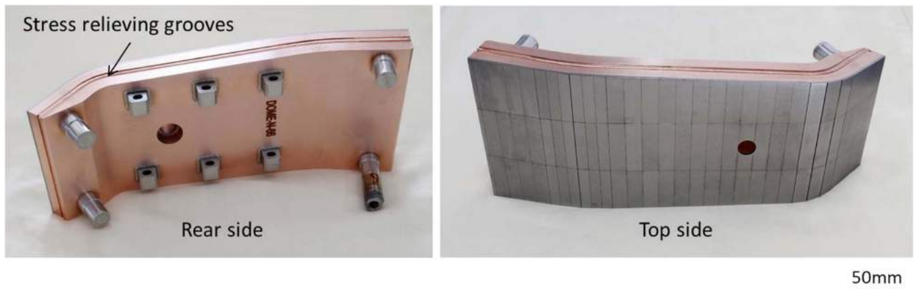
Figure 13. Dome component for EAST upper divertor consists of two parts, namely upper W/Cu plate and lower CuCrZr plate, which are assembled by EBW.
