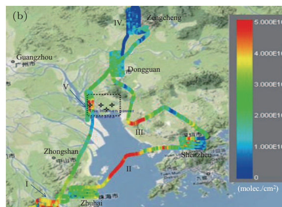
Fig. 4. (color online) (a) Time series of \text{NO}_2 slant column densities for AMAX-DOAS on 10 December 2008 in nadir and zenith directions. Four strong enhancements (I, II, III, and V) and one decrease were detected. (b) \text{NO}_2 vertical column density distribution along the flight track. The Humen power plant area is indicated by the black rectangle where stars stand for the location of its chimneys.
