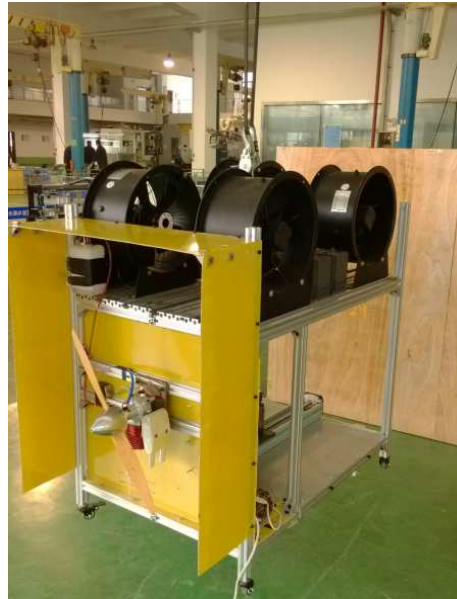
Fig. 2 Suspended fire fighting robot prototype
