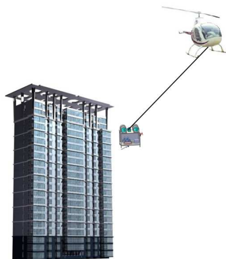
Fig. 1 Suspended fire fighting robot working principle diagram
