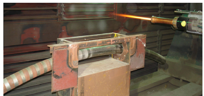
Fig. 7. Picture of HVOF thermal spraying of Cu coating on Inconel 625 tube used in EAST in-vessel cryopump.
