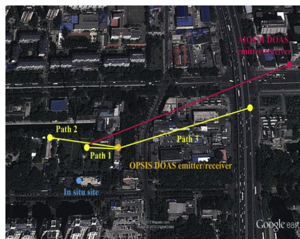
Fig. 1. Measurement site with instrument positions, three OPSIS DOAS paths in different directions and one AIOFM DOAS path. The topography is captured from Google Earth.
