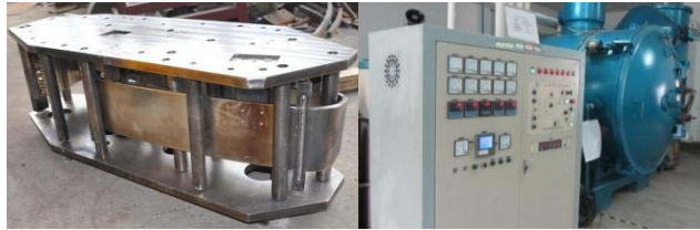
Fig. 8. Status of the central conductor after heat treatment (left) and vacuum furnace for heat treatment (right).
