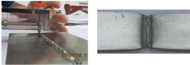
Fig. 3. Permeability inspection (left) and tensile test (right) of the weldment.
