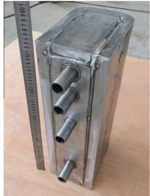
Fig. 13. 1/3 Scale ITER DFLL-TBM fabricated with CLAM steel.
