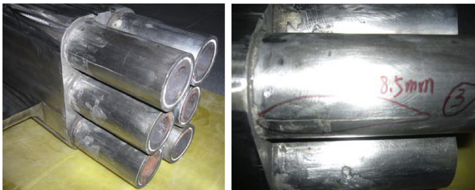
Fig. 12. The cracks in the jacket surface.
