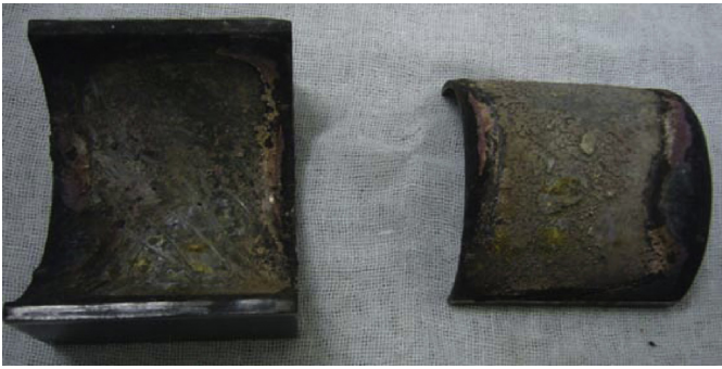
Fig. 4. The experiment result of bracket sample with the pure powder as the filler.
