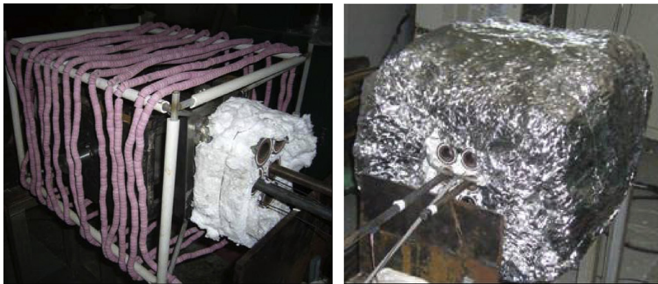
Fig. 9. The heating oven assembly process for bracket brazing.
