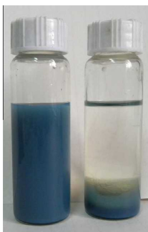
Fig. 4. Digital photographs of modified (a) and pure (b) ITO NPs dispersed in urethane acrylate oligomers.
