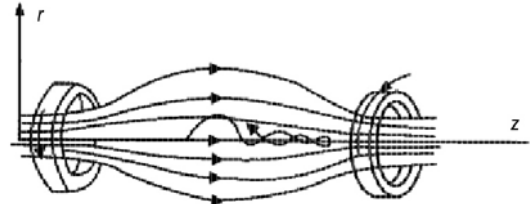
Fig.9 Principle drawing of the magnetic mirror
