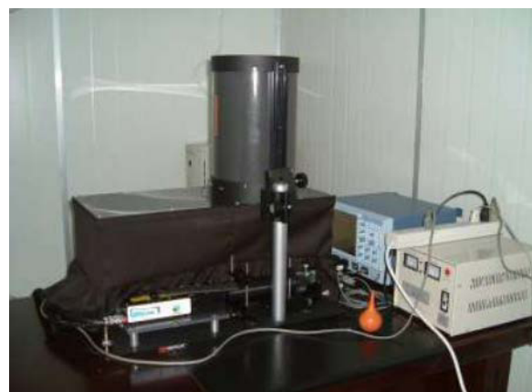
Fig. 1 Two-wavelength depolarization lidar initialized in SKYNET Hefei site by NIES, Japan
