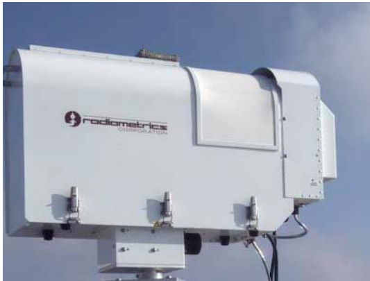
Fig.2 Two-band microwave radiometer installed in Hefei by SKYNET
