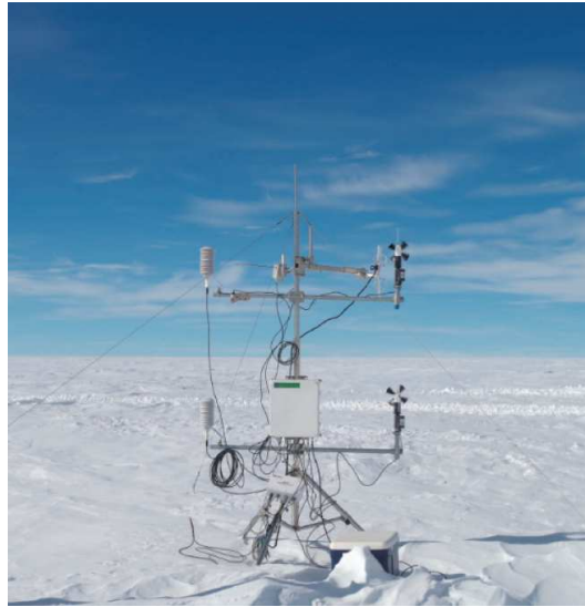
Fig. 1. Mobile atmospheric parameter measurement system over snow and sea ice at Antarctic Taishan Station.
