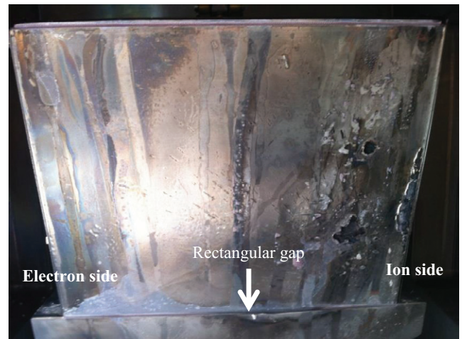
Figure 7. The picture of the FLiLi limiter surface taken in the air after the campaign of EAST.
