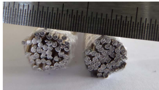
Fig. 1. Bi-2212 cable (left: before compaction, right: after compaction).
