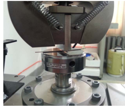
Fig. 4. The process of artificial indentation is applied on a Bi-2212 strand.
