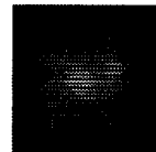
Fig.2 Far-field spot of oscillator output
