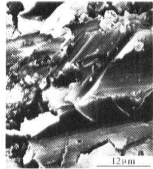
图5 未增韧的F体系在4.2K下的断面形貌 Fig.5 SEM from the fracture area of non-toughening A resin system at 4.2K
