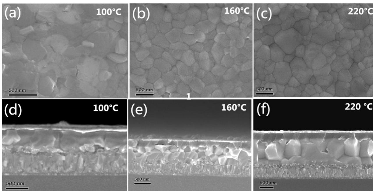
**Fig. 3.** The surface morphology and cross sectional SEM images of perovskite solar cells prepared at different temperature, (a) and (d) 100 °C, (b) and (e) 160 °C, (c) and (f) 220 °C.
