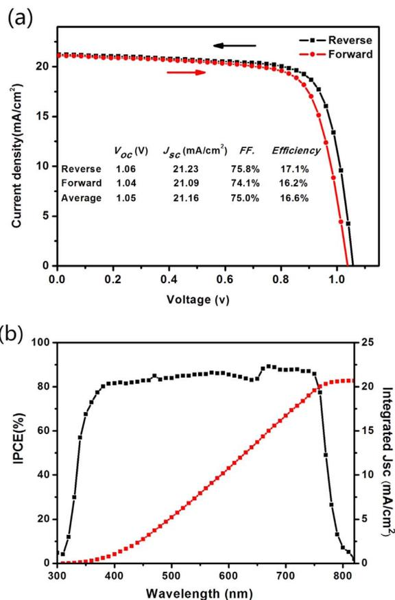
Fig. 6.  $J$ - $V$  and IPCE characteristics for the best cell obtained in this study. (a)  $J$ - $V$  curves of forward and reverse bias sweep for the solar cell (b) corresponding incident photon-to-current conversion efficiency (IPCE) and integrated  $J_{sc}$  spectra.
