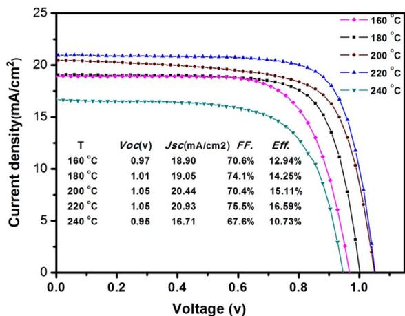
Fig. 5. The photovoltaic performance of the devices prepared by different annealing temperature (160 °C, 180 °C, 200 °C, 220 °C, 240 °C) were measured under simulated AM 1.5 G (100  $\text{mW}/\text{cm}^2$ ) solar irradiation in air, which was calibrated using a certified monocrystalline silicon solar cell.
