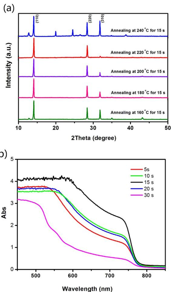
**Fig. 2.** (a) XRD patterns of perovskite films deposited on glass substrate treated by different temperature (b) UV absorption of perovskite film annealing at different time deposited on meso- $\text{TiO}_2/\text{TiO}_2/\text{FTO}$  substrates.
