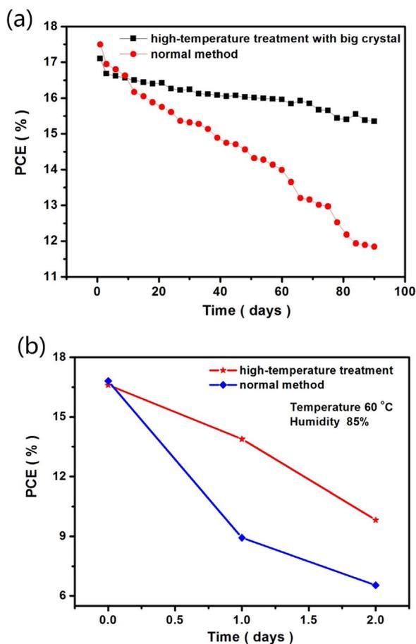
**Fig. 7.** The performance of perovskite solar cell prepared by high-temperature treatment and normal method. (a) Power conversion efficiency as a function of storage time in dry air and dark conditions for the perovskite solar cell with different method, the test time interval was three days (b) two type devices was stored in Humidity Chamber under the condition: temperature of 60 °C and humidity of 85%.
