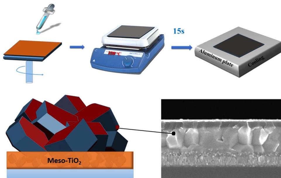
**Fig. 1.** Schematic of high temperature treatment for Perovskite solar cell rapid preparation and large particles crystals prepared by high temperature-induced method. Low temperature aluminum as heat transfer plate to prevent the film from continuous heating.
