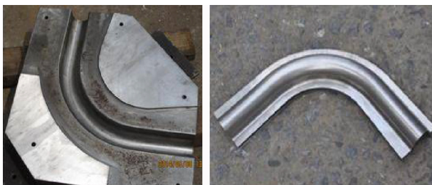
Fig. 3. Punch tool and part of omega shape compensator.
