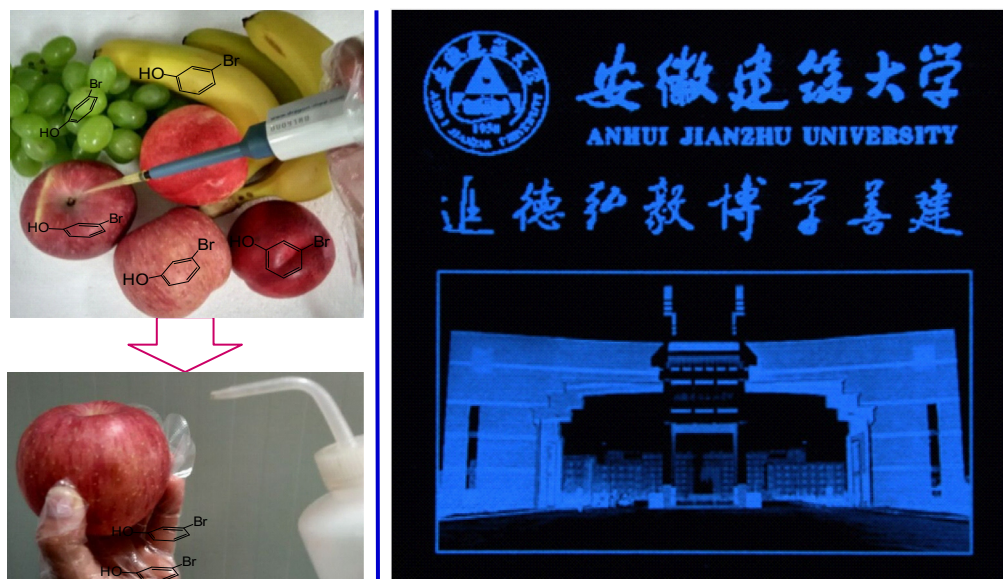
Fig. 6. A lab-leveled mimetic insecticide residuals method to synthesize C-dots as colorless inks (left). Printed patterns obtained by C-dots ink and imaging under 365 nm UV lamp.
