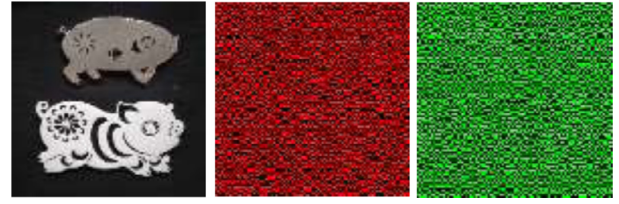
Fig. 3. Experimental illustration: on the left are the objects, and on the center and right are the encoded matrices. The encoded matrices are 128 \times 128 binary matrices, which contain 8192 elements equal to 1 and where different colors represent different polarization states. The compression ratio is 50%.
