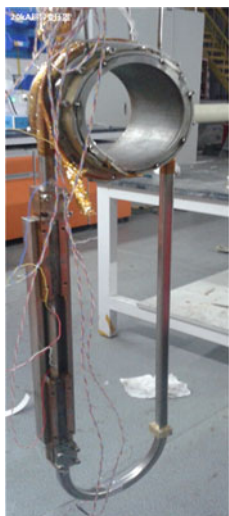
Fig. 8. Assemble conductor sample for I_c test at self-field and Liquid He.
