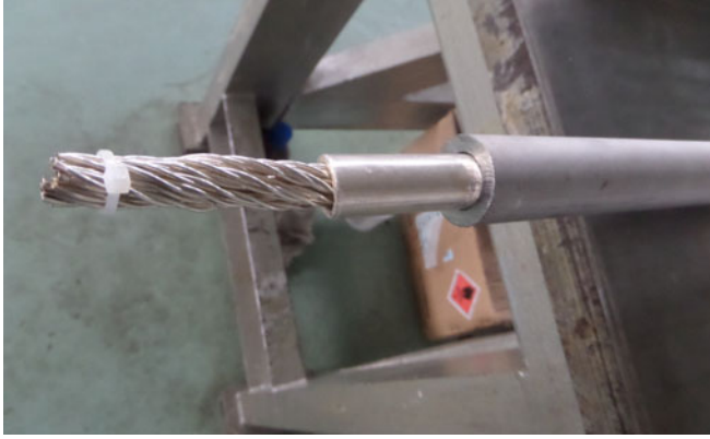
Fig. 5. Photo of manufactured Bi2212 conductor with SS jacket outside and Ag tube in between.
