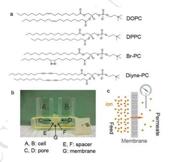
Fig. 1 Chemical structures of lipids and images demonstrating the diffusion unit and process. (a) Molecular structure of lipids DOPC, DPPC, Br-PC and Diyne-PC. (b) Digital photo of the diffusion unit, including cells (A, B) with pores on one side (C, D), spacers (E, F) with pores, and the sandwiched membrane (G; cannot be seen here). Another spacer (and membrane) was
