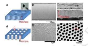
Fig. 2 Schematic and SEM images of the MWNT- (a-c) and AAO-CT- (d-f) membranes. (a) Schematic, (a-inset) digital and (c) cross-sectional SEM images of a MWNT-membrane. (b) presents the aligned MWNT array grown vertically on a substrate. (d) Schematic, (e) cross-sectional and (f) top-view SEM images of an AAO-based amorphous CT-membrane.
