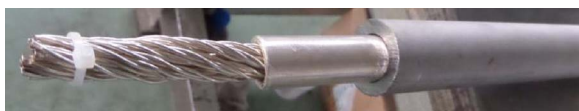
Fig. 1. Photo of manufactured Bi2212 conductor with SS jacket outside and Ag tube in between.
