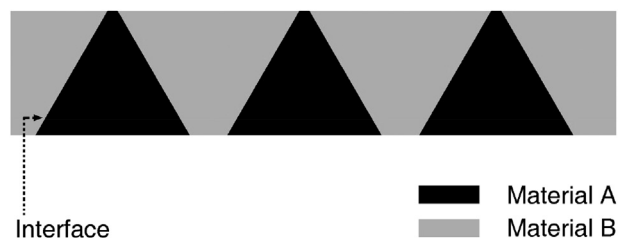
Scheme 1. The schematic design for the thermal rectifier composed of two different materials with asymmetric shape and interfaces.
