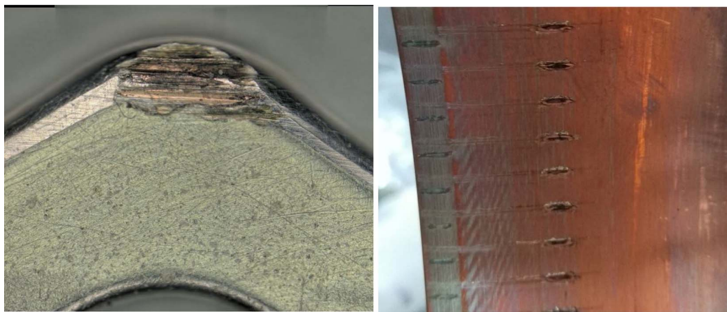
Fig. 16. Left: zoom on the tip of louver after 30 000 cycles. The wearing of the louver is of the order of 150 µm. Right: Picture of the CuCrZr ring after 30 000 cycles. The 1.5 mm long scratches depth (in the middle of the picture) is of the order of 60–80 µm on a width of 0.1 mm.
