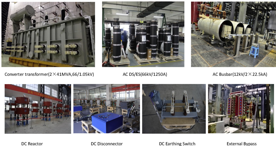
Fig. 8. Manufacturing of each component and the system integration.
