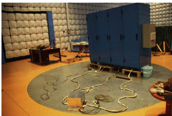
Fig. 10. The EMI and EMC tests site of local controllers.
