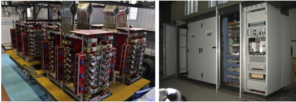
Fig. 6. The prototypes of converter module and local controller.
