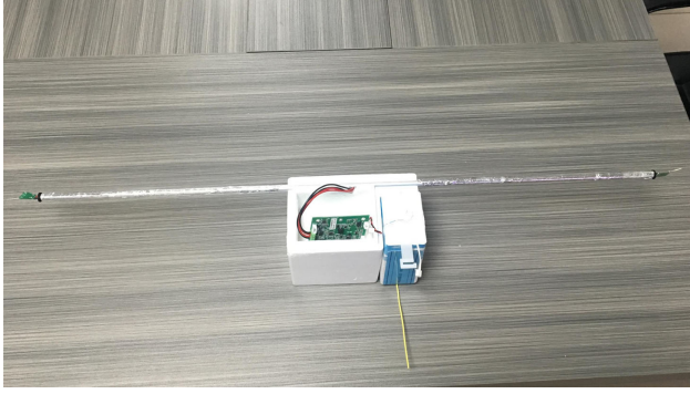
Fig. 3. Equipment of micro-thermometer used in balloon-borne radiosonde.
