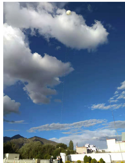
Fig. 2. Balloon-borne radiosonde is launched at Lhasa Meteorological Station.
