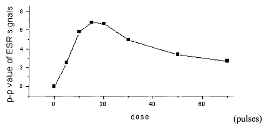
Fig. 4. The variance of radical concentration in irradiated glycine at different dose the sample was irradiated with 30 keV nitrogen ion at room temperature and the EPR spectra were recorded at room temperature after the sample was kept at room temperature for about 15 h.
