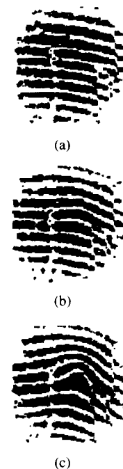
Fig. 8. Interferogram data on optical path difference measurements in the \text{AgGaSe}_2 OPO crystal at various pump power levels. Changes in the fringe pattern show weak thermal lensing with increasing pump power: (a) pump beam blocked; (b) 1.2-W incident pump power; (c) 2.25-W incident pump power.
