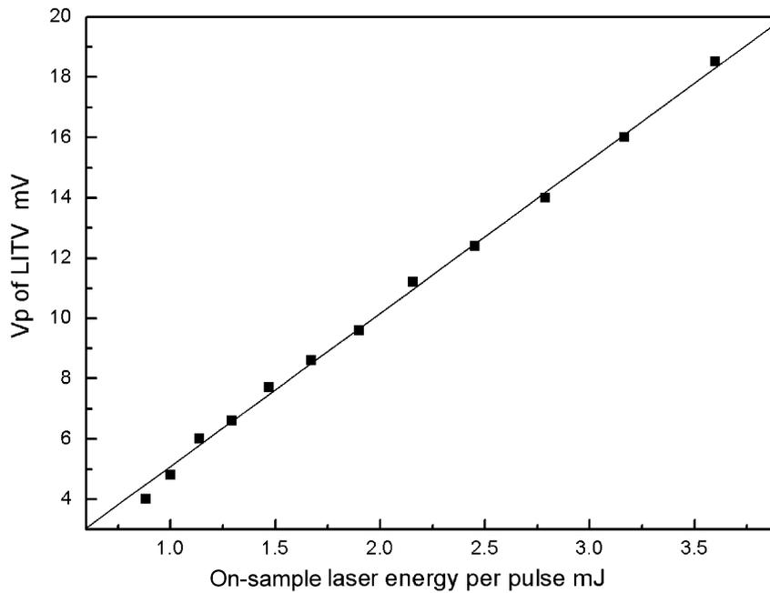
Fig. 2. The linear relationship between peak voltage  $V_p$  and the on-sample laser energy per pulse for  $\lambda = 1064$  nm. The solid line is a guide for the eye.
