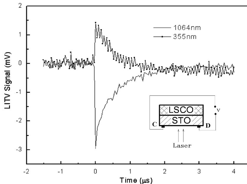
Fig. 3. Voltage signal as a function of time under irradiation of 355 and 1064 nm laser, respectively, on the STO substrate. The inset shows the schematic circuit of the measurement and irradiation direction.
