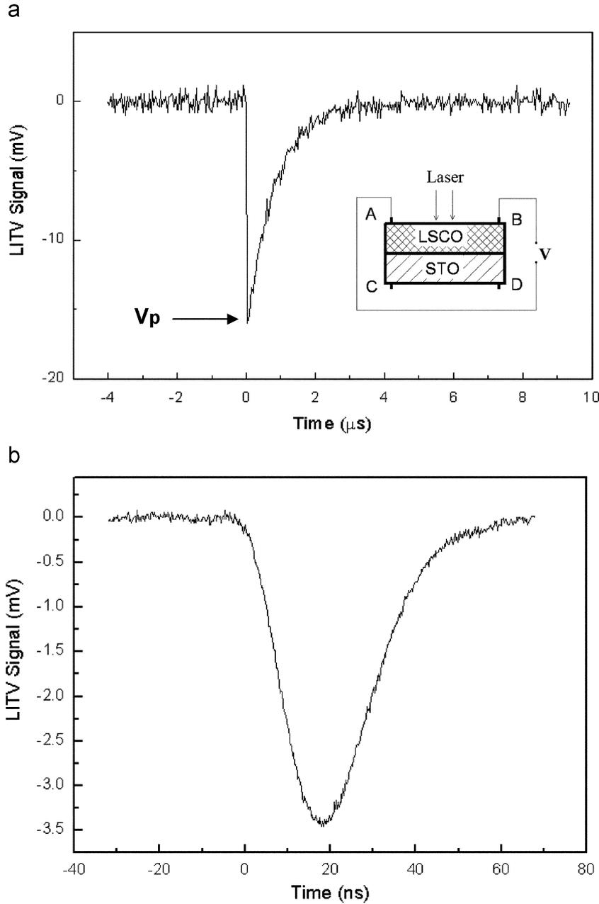
**Fig. 1.** (a) The inset shows the contact arrangement of the sample and the schematic circuit of the measurement. A typical voltage signal measured on electrodes A and B when the LSCO film was illuminated by 1064 nm laser with 1 MΩ and 50 Ω and (b) input impedance to oscilloscope.  $V_p$  is the peak voltage.
