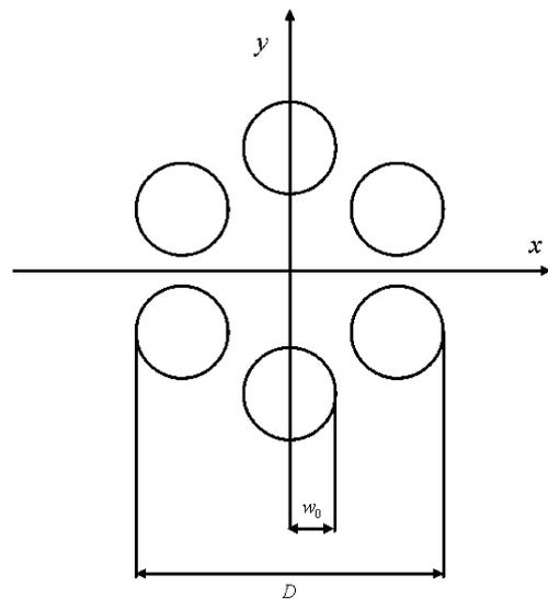
Fig. 1. Schematic diagram of the radial laser beam array.
