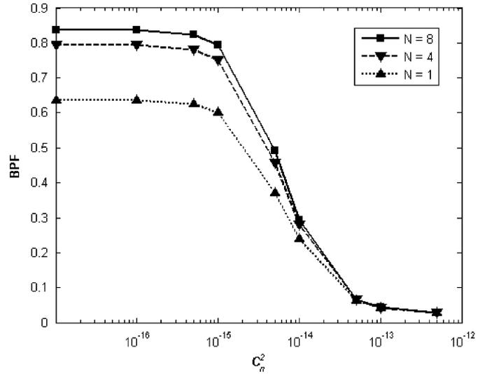
Fig. 3. The dependence of BPF on the intensity of turbulent atmosphere.
