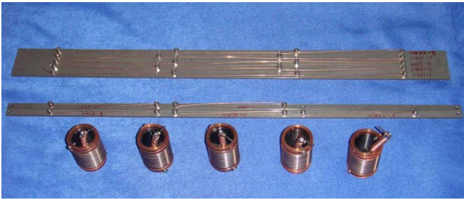
Fig. 2. Preparation of the superconducting strand samples before the HT. (Top) Straight samples for RRR tests. The coils at the bottom were used in the I_c measurements and hysteresis losses.
