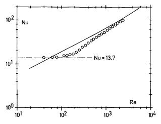
Figure 4. Mixed convective heat transfer in pebble beds under opposing flow conditions.
