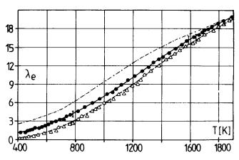
Figure 14. Effective conductivity of packed beds in vacuum and helium. Experiments and theory after Ref. 33; - - 22.
