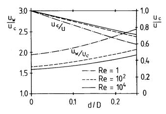
Figure 12. Ratio of wall-to-center and center-to-mean velocities.
