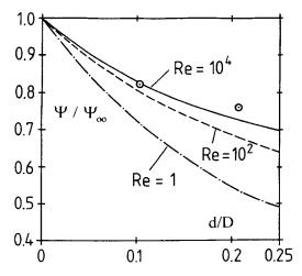
Figure 13. Effect of bypass flow on the pressure drop coefficient. ( $\odot$ ) Present experimental result. Re = 10<sup>4</sup>.
