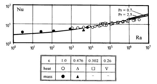
Figure 3. Natural convective heat/mass transfer in pebble beds; solid lines: Eq. (20).
