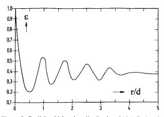
Figure 8. Radial void fraction distribution. (After Ref. 11.)
