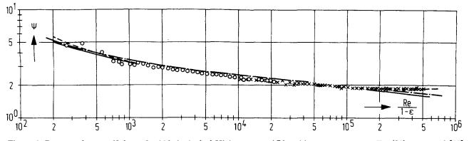
Figure 6. Pressure drop coefficient of pebble beds. ( $\times$ ) High pressure, ( $\bigcirc$ ) ambient pressure. — Eq. (21), — ref. [22].
