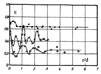
Figure 11. Radial void fraction distribution. Ref. 14: ring ( $\bigcirc$ ),  $d_i/d_a = 0.67-0.77$ ; full cylinder ( $\bigcirc$ ). Ref. 16: ring ( $\times$ ),  $d_i/d_a = 0.425$ .
