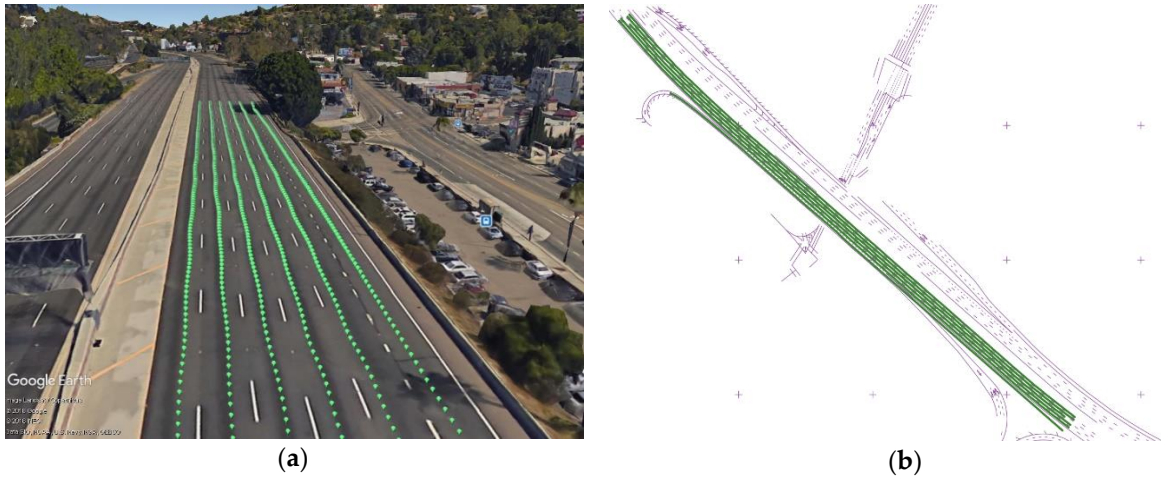
491 Figure 12. Extraction of the lane's centerline: (a) Extraction results obtained by Google Earth; (b) Shapefile of 492 the US101 highways.
